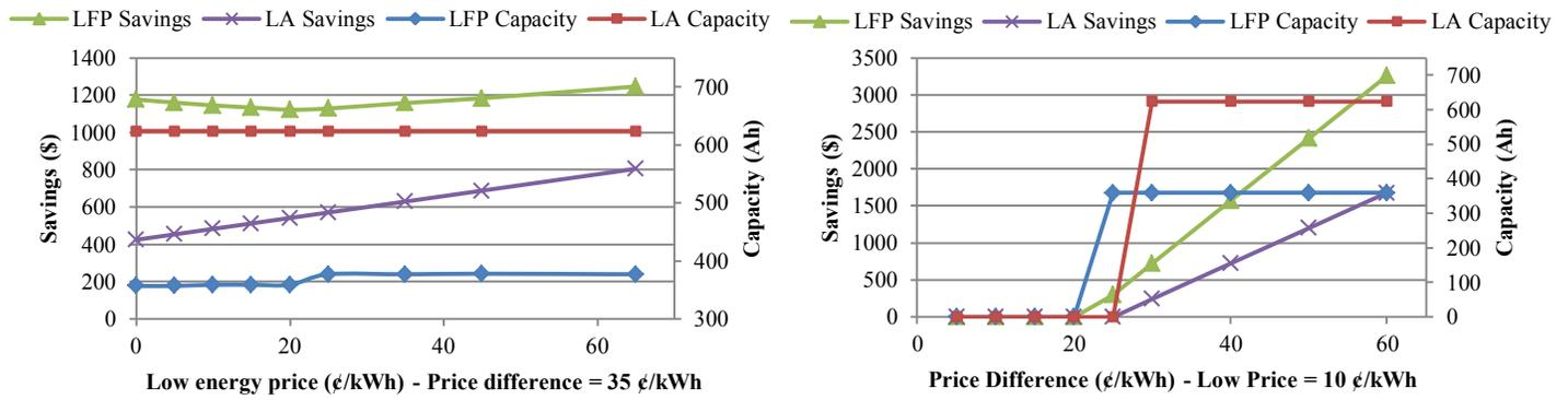
Fig. 6. Savings&capacity vs. price differences using House 1 power profile. a) Fixed 35 €/kWh price difference with changing low energy price, b) Increasing price difference with fixed 10 €/kWh low energy price
