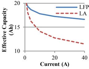
Fig.1. Effective capacity of 20Ah LA & LFP batteries
