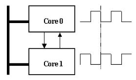
Fig. 6. Cores with non-overlapping active times.
