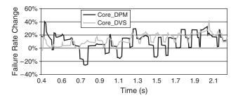
**Fig. 7.** 2-core system, Core0 with DPM, Core1 with DVS; both running a higher utilization trace.
