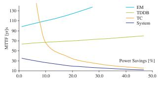
Fig. 1. Failure mechanisms in 95 nm technology for a single core.
