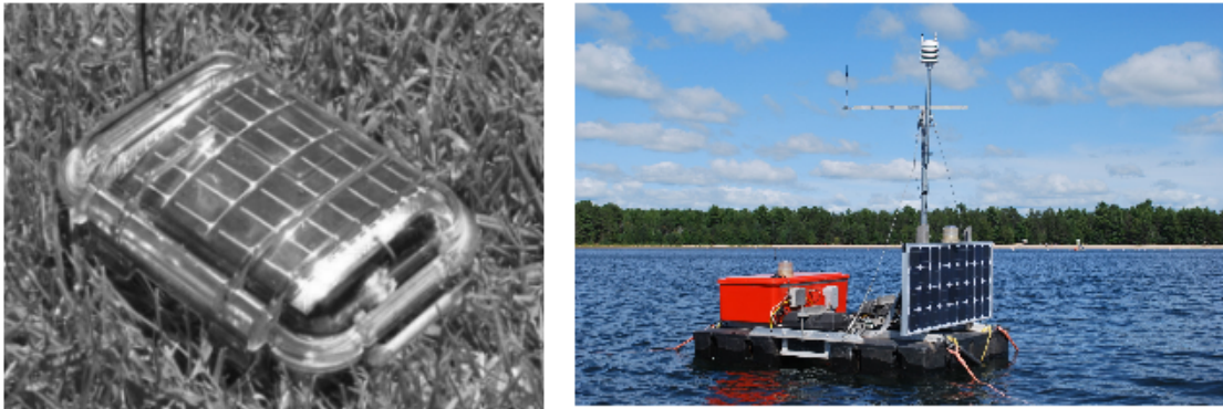
Figure 1.1: Environmental monitoring sensing platforms, (left) Heliomote [33] (right) Buoy deployed in a lake located in northern Wisconsin, USA measuring several key limnological variables [68]
