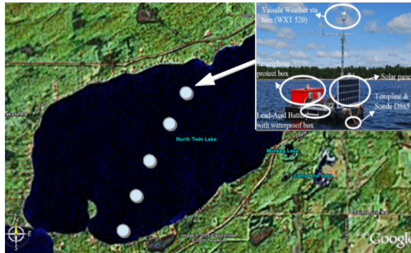
Figure 3.7: Example of linearly deployed buoys in a single lake [69]
