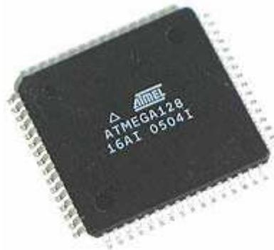
**Figure 3.14 – Atmel ATmega128 in TQPF package.**
