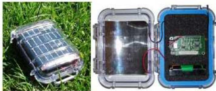
**Figure 2.19 – The energy harvesting module Heliomote.**
