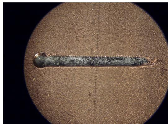
**Figure 5.4 – Imperfections caused by milling tools' deterioration.**
