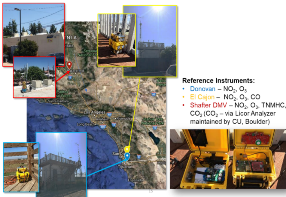
Figure 3. Map and images of deployment locations. Shafter DMV (red) was located 250 mi away from Donovan (blue) and El Cajon (yellow), which were located in San Diego, CA. (bottom right) Deployment containers configuration for the extended deployment. Each container has active ventilation to keep the internal conditions equivalent to the ambient environment.
